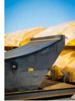
CBE Group's expertise is based on its ability to design a long-lasting mould which will produce a high quality segment. Each mould is designed to produce at least 1,500 segments.
