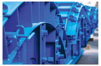
CBE Group has successfully taken part in the development of **segment moulds for tunnels of all dimensions:** 1 to 17 m diameter, 18 to 60 cm thickness, 3 to 17 tons.
